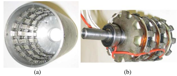
Fig. 1. Prototype of a PM TFM, (a) PM rotor, (b) 3 stack SMC stator
